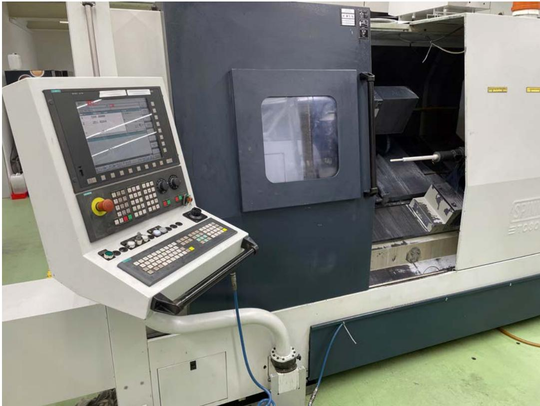
**Universaldrehmaschine | Universal lathe**
